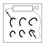
In order to probe the circuit you need to connect the red clip to a wire and the blue clip to a different wire. Common frequencies in both wires will cancel out and the display will show the remaining frequencies, in order from lowest to highest.
