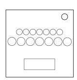
Press the button when the top LED and the corresponding LED in the bottom row are both lit. Repeat this until all LEDs are lit.
